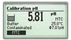
Electrode Dirty/Broken alternatively with Buffer Contaminated –The offset of the electrode is not in the accepted range. Check if the electrode is broken or clean it following the Cleaning Procedure at the end of this section. Check the quality of the buffer. If necessary, change the buffer.
