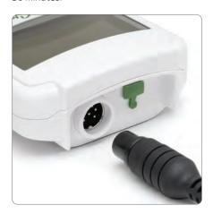
Each meter features an application specific pH/temperature probe with a quick connect DIN connector to make attaching and removing the probe simple and easy.
