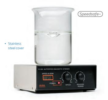
When stirring a solution, to work with a constant speed is an important factor in ensuring that the best repeatability in tests and processes is achieved. Without a tachometer, there is no way of knowing the RPMs.
