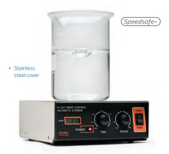
HI324N is a heavy-duty stirrers that incorporate a timer control that will turn the motor off after a selected amount of time. The time is adjustable from 5 minutes to 2 hours. This feature allows the user to carry out other tasks without worrying about over or under stirring. HI324N can stir up to 5.0 liters (1.3 gallons), making it ideal for laboratory and production use.
