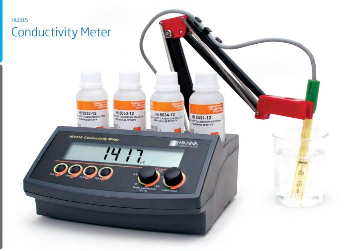
The HI2315 is a basic and affordable conductivity benchtop meter that comes with a four-ring potentiometric EC probe with a built-in temperature sensor. Operation of the meter is simplified to calibration, range selection, and adjustment of the temperature compensation coefficient.
